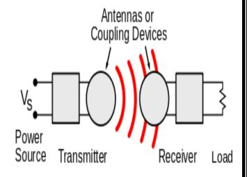
Wireless power transfer is a generic term for a number of different technologies for transmitting energy by means of electromagnetic fields. The technologies differ in the distance over which they can transfer power efficiently, whether the transmitter must be aimed (directed) at the receiver, and in the type of electromagnetic energy they use: time varying electric fields, magnetic fields, radiowaves, microwaves, infrared or visible light waves.
